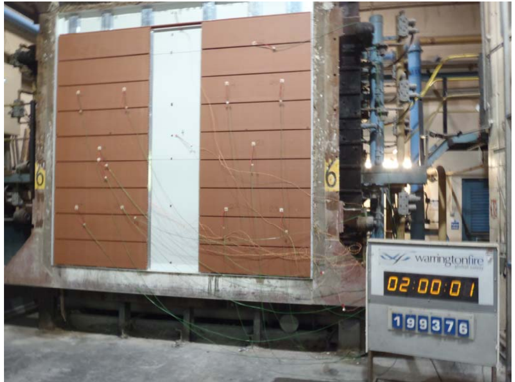
The unexposed face of the test construction after a test duration of 120 minutes
