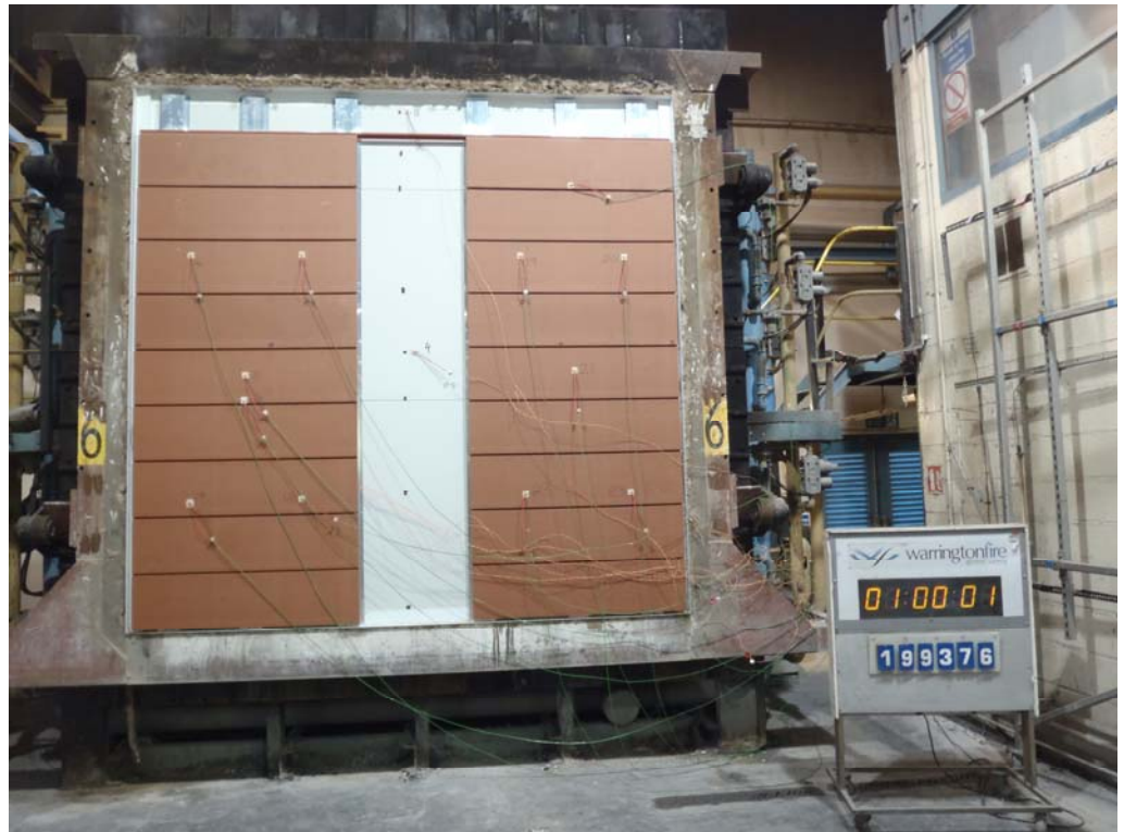
The unexposed face of the test construction after a test duration of 60 minutes
